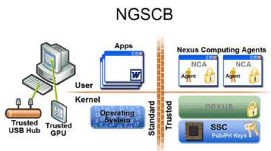
Fig 1: curtained execution in NGSCB-enabled system.
