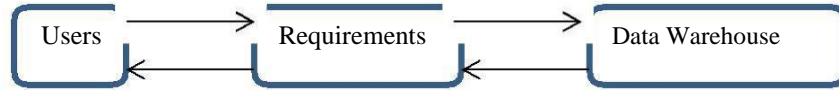
Figure 3: Forward and backward traceability links from data warehouse users to the data warehouse
